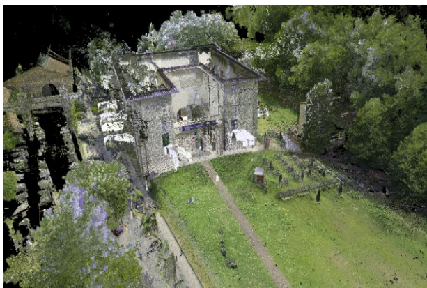
Figure 3. Point Cloud Generated from Laser Scanner Data Processing for the Valorisation of the Medici Villas and Their Context
