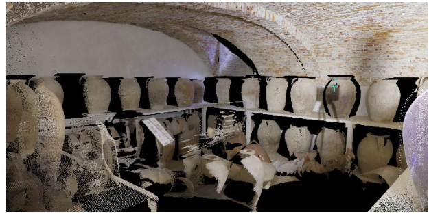
Figure 4. Point Cloud Generated from Laser Scanner Survey of the Interiors of the Medici Palace in Seravezza: Room for the Exhibition of the Medici's Ancient Jars"
