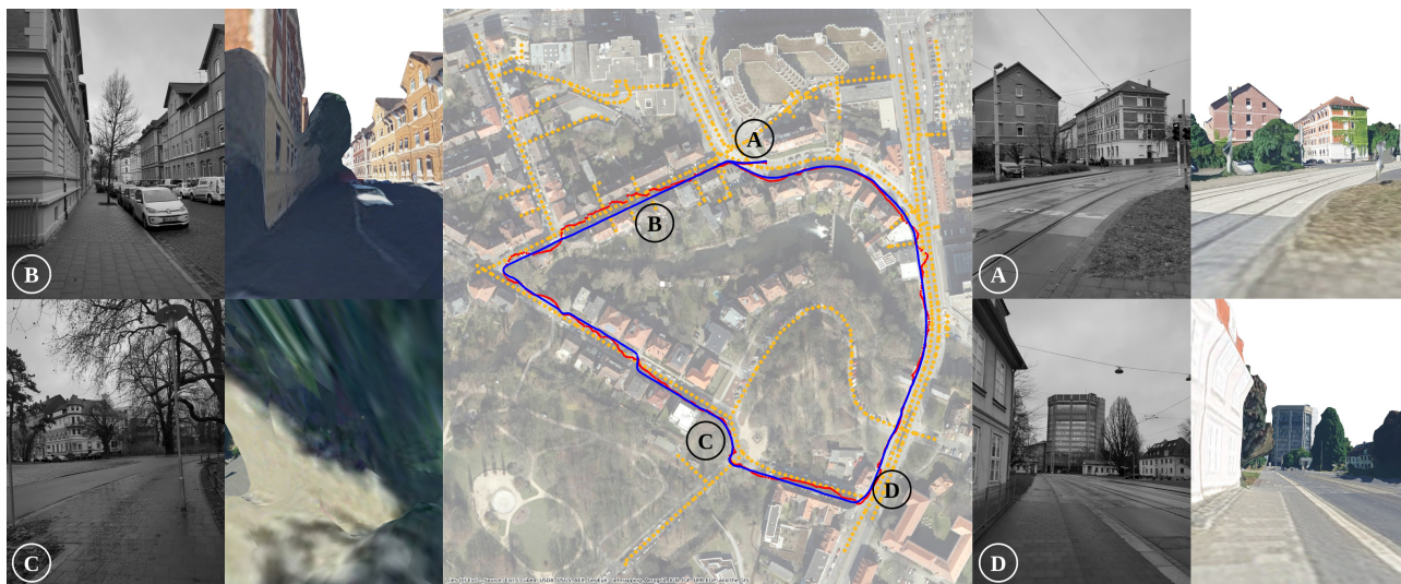
Figure 2. In the center, the reference trajectory of the camera in blue, the smartphone’s internal GNSS pose estimate in red, and the sampled views in orange, over imposed to a satellite image of the area. On the left and right side we show four examples of the query images and the view rendered from its reference pose
