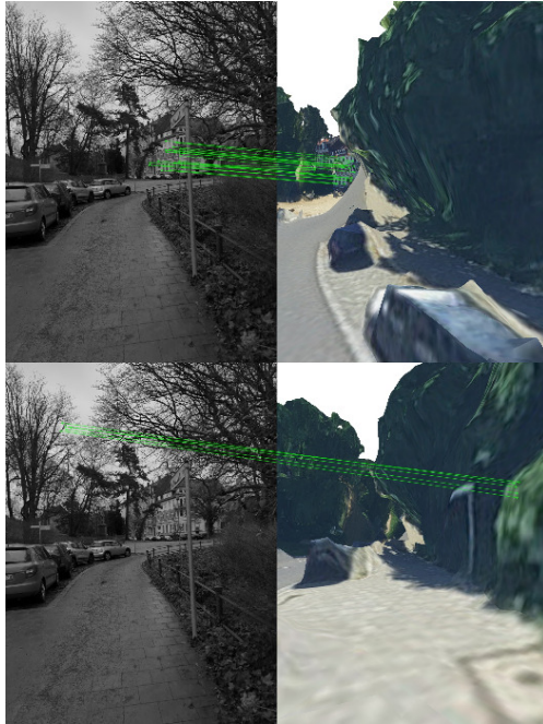
Figure 4. Comparison of feature matches between the query image \mathcal{I}_q and an image rendered from the best pose (top) as determined by SNN-LFr, showing successful matching, and an image rendered from the reference pose (bottom), only spurious matches were found. Both examples use XFeat and Lighter Glue for image matching.
