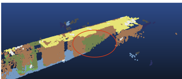
Figure 5. Example of a wall mislabeled as a door due to labeled mesh inaccuracies in Office 10s .
