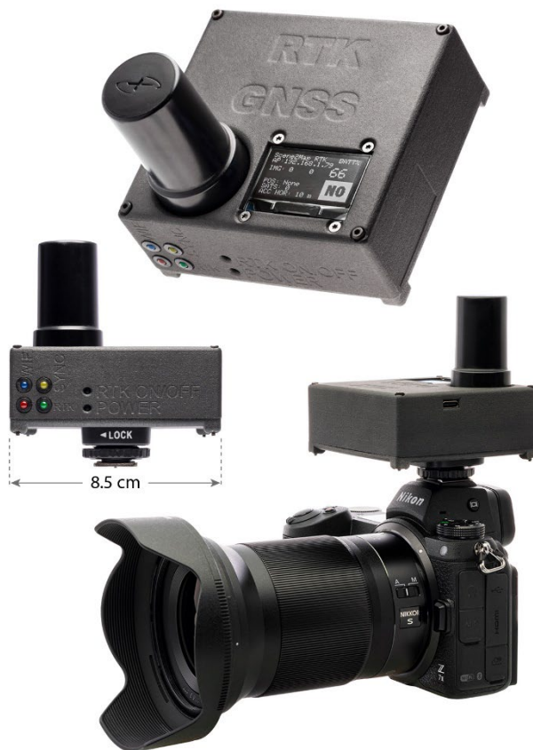
Figure 3. The RTK-enabled GNSS/IMU logging device. The lower inset shows the device on top of the Nikon Z7 II.
