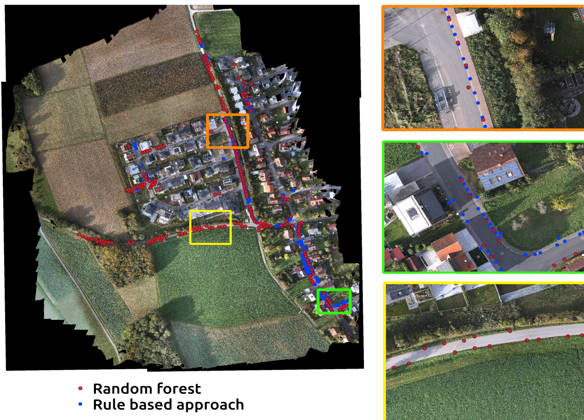
Figure 7. Predicted curb points using the rule-based and random forest approaches. The rule-based approach produced more accurate predictions compared to the random forest approach, further, with higher point density as can be seen in the orange and green boxes. The random forest approach showed a higher number of wrongly assigned curb points (red box).
