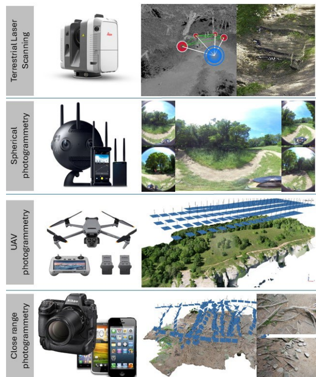
Figure 2. The most widely used geomatic technologies for soil erosion monitoring.
