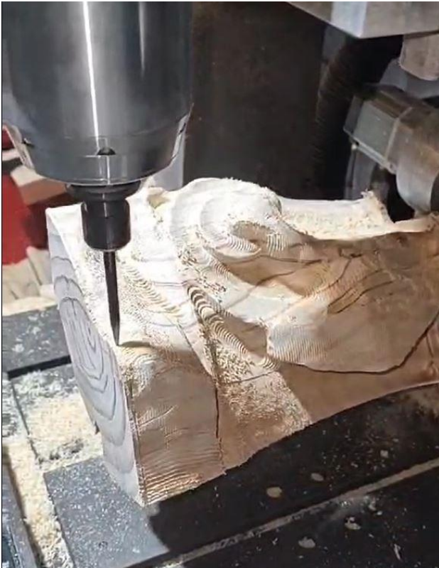
Figure 6. Phase two of prototyping, semi-finishing step.
