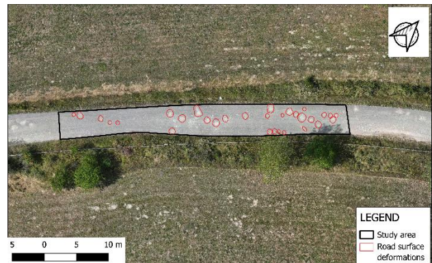
Figure 9. Road surface defects affecting the analysed road section.
