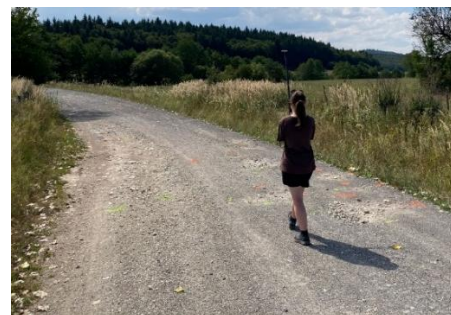
Figure 4. Collection of near-nadir images from a height of approx. 2 meters, using a GoPro Hero 10 action camera mounted on a monopod.
