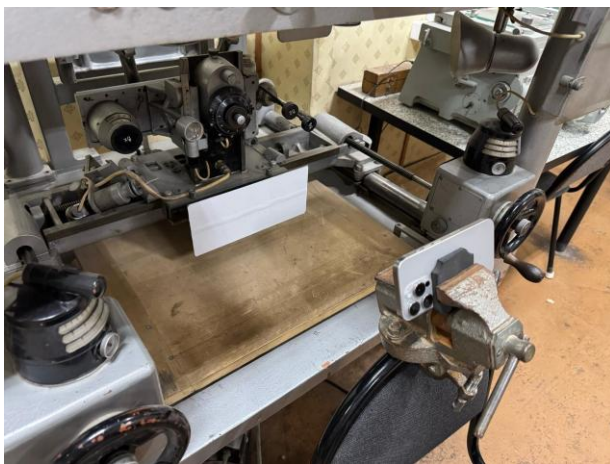
Fig.5 Capturing the plate with a fixed smartphone camera tilted in relation to the plate
