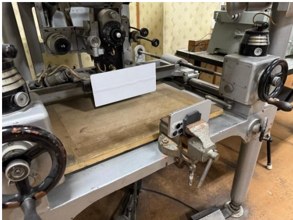
Fig.3 Capturing the plate with a fixed smartphone camera
