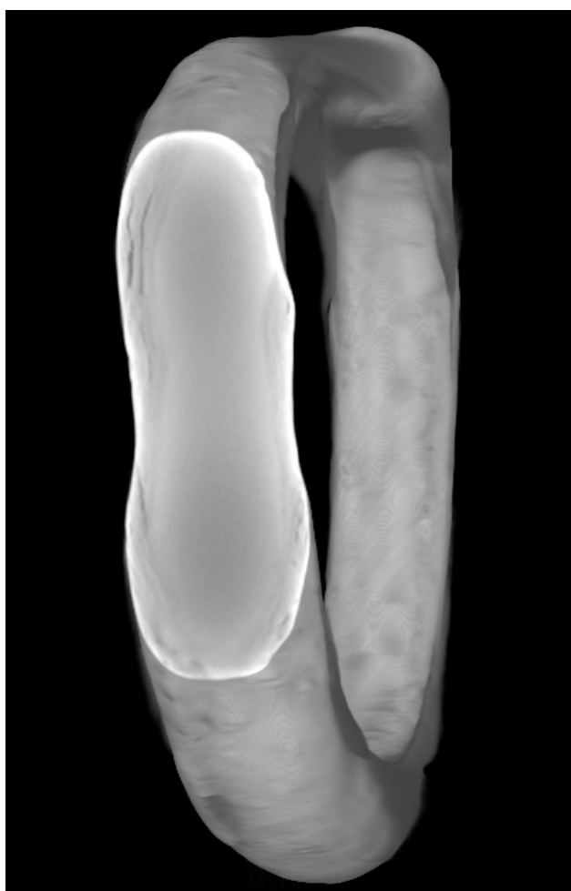
Figure 7. "Cut" CT image of the bronze bracelet. Layered texture is clearly visible.
