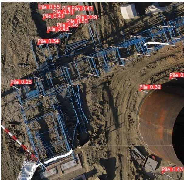
Figure 8. Example of pile recognition results on an orthophoto
