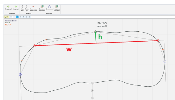
Figure 6. Contour with marked width (w) and height (h) of vestibular (labial) contour segment.
