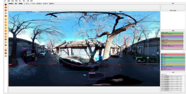
Figure 2. Label the categories of images using X-AnyLabeling and generate annotation files in COCO format.
