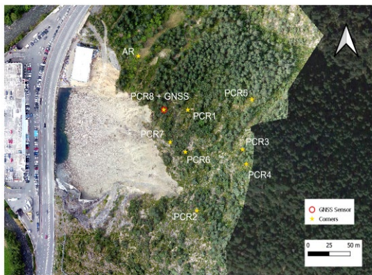
Figure 2. Map of collapsed area and the locations of the different artificial reflectors.
