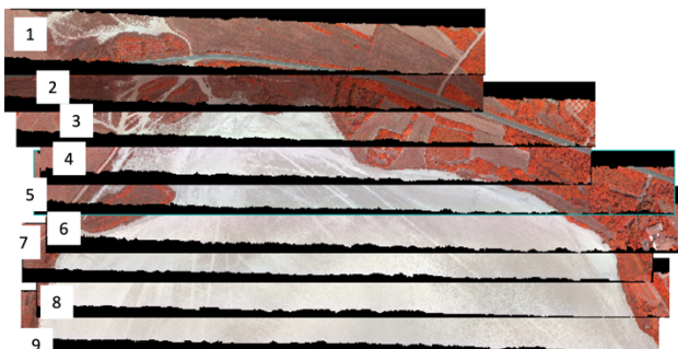
Figure 9. Line 1-6 acquired 20 July and lines 7,8,9 on 18 July 2023 raw data processed in CaliGeoPro, by Specim. DN processed as raw data – dark current, then into radiance Georeferenced AISA data file radiometrically corrected to radiance (mW/cm 2 *str*um)*1000.00
