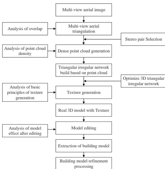
Figure 3. The process of Real 3D model construction.
