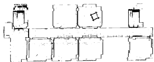
Figure 11. Wall line point cloud
