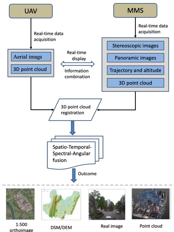
Figure 3. The combination of UAV and mobile mapping vehicle system.
