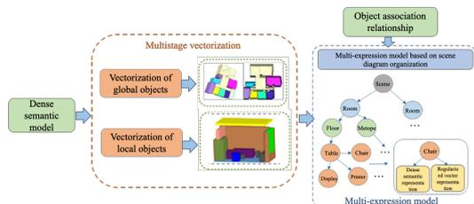
**Figure 7.** Schematic diagram of indoor multi-expression model construction
