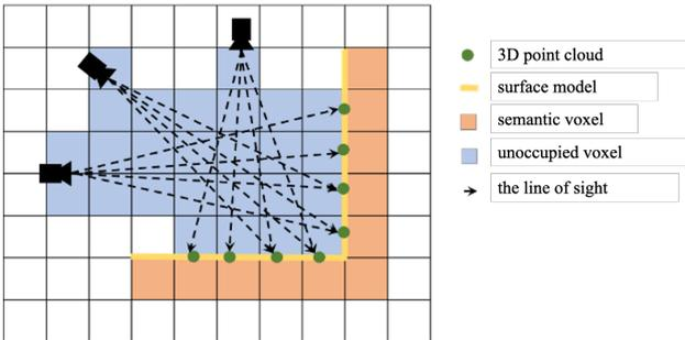
**Figure 6.** Two-dimensional diagram of voxel segmentation.
