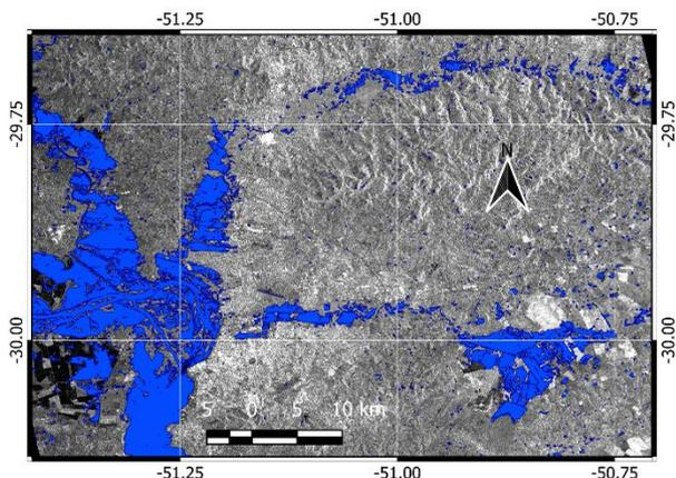
Figure 7. Flood curve classification map shown in blue, with the Lessônia SAR radar image in the background.
