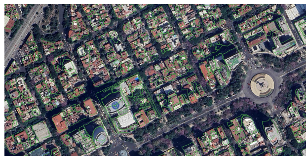
Figure 6. The building footprints that were created using the INEGI data. By taking advantage of the DSM data and not enforcing strict rectilinear polygons, the method creates reasonably accurate building footprints for complex buildings.
