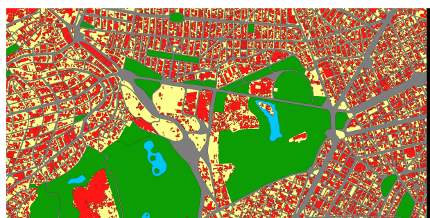
Figure 7. The polygons that are lifted: roads, building footprints, plant cover, water bodies and terrain.
