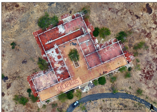
Figure 6. Orthophoto of the Officers' Club (Casa de Piedra) clearly reading from above Galapagos Service Club, derived from 78 images taken at 65 m from the ground and mosaicked using Drone2Map.
