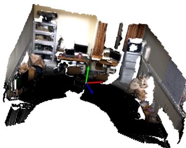
Figure 2. The HoloLens 2 local cloud is defined relative to the spatial coordinates of the device, with the location of the device serving as the origin.
