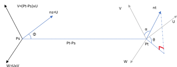
Figure 3. Creating the point features frame from two points for computing the PFH
