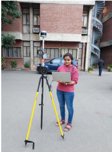
Figure 2. Data Collection using VLP 16 Sensor.
