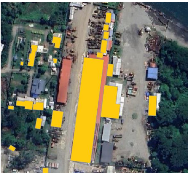
Figure 5: Placement inaccuracy of the building footprint shapefiles used to create the spatial Digital Twin.
