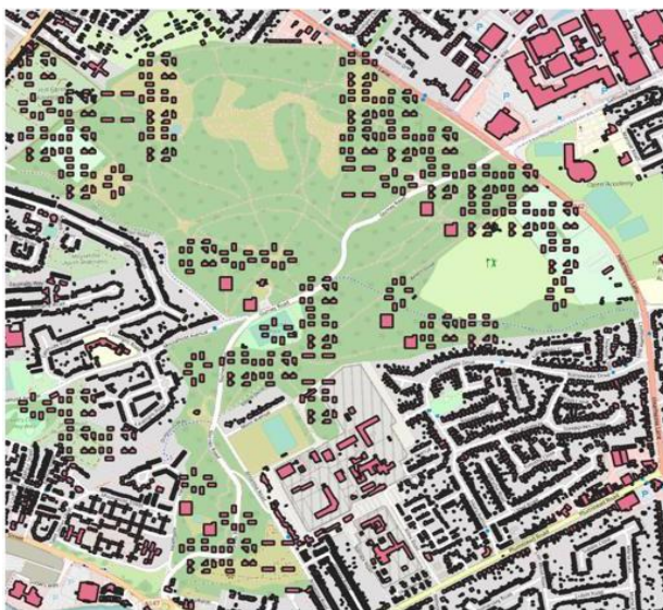
Figure 7: UFG generated 2080 buildings amalgamated with existing urban digital map data for the city of Norwich.
