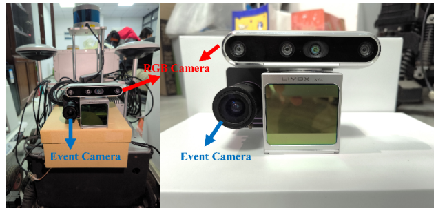
Figure 4. Setup of event camera and RGB camera mounted on a wheeled robot.
