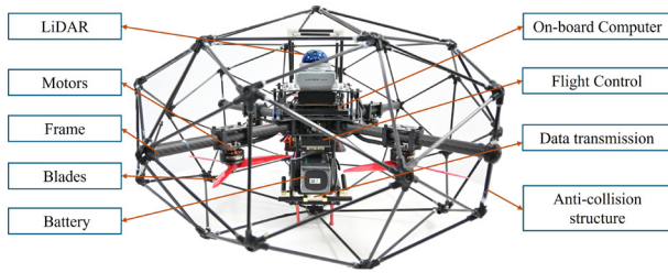
Figure.1 Hardware System of LUOJIA Explorer UAV
