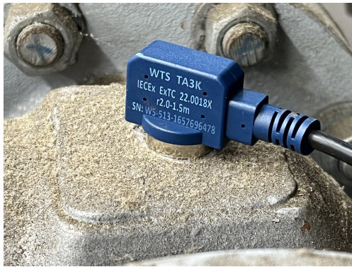
Figure 3. An accelerometer sensor attached to equipment
