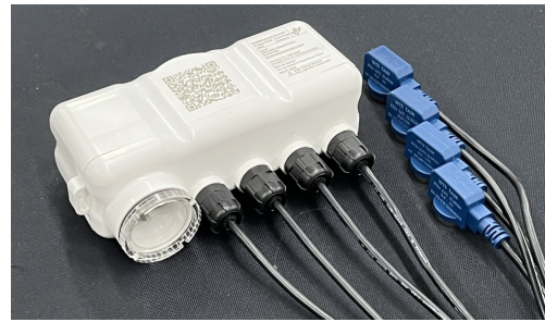
Figure 1. An IoT device with four accelerometer probes attached with magnetic accelerometer sensor probes attached (to measure vibration for purposes of condition monitoring) is shown in Figure 1.
