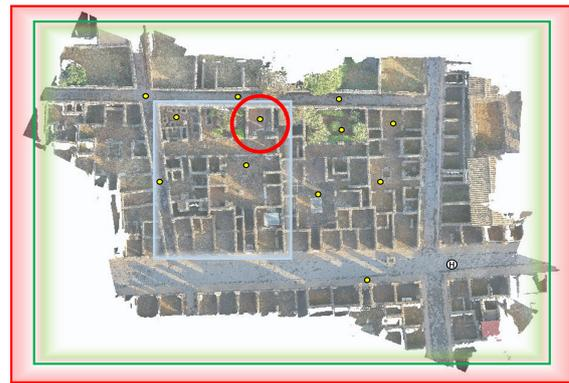
Figure 3. Schema of integrated survey campaign. UAV photogrammetry at 40 m AGL was performed over red areas, UAV photogrammetry at 15 m AGL was conducted over green areas, whereas laser scanning and terrestrial photogrammetry surveyed the light blue areas, respectively. The red circle represents the room where the data processing is focused.
