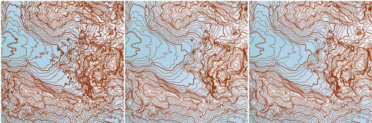
Figure 5. Exemplary result of contour line derivation around the two Ushba peaks (right centre) and the Ushba Glacier. From left: unmodified DSM, multiple low-pass filtered DSM, smoothed using polynomial method. Scale 1:80,000, equidistance 50 m.
