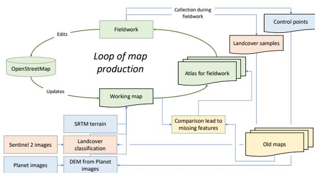
Figure 3. The use of dynamic working map and field atlas in the process of updating and augmenting geodata.
