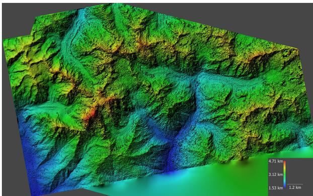
Figure 4. Colour-coded DSM calculated from 11 PlanetScope scenes from Jaspersen (2021).
