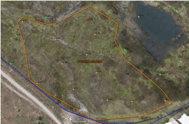
Figure 9. 2020 RPAS survey digital elevation model compared with prior 1:2.000 digital elevation model (1999) for the south west area subjected to negligible height changes between 1999 and 2020.
