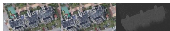
Figure 2. The WHU dataset for training, test, and validation. From left to right: stereo-left image, stereo-right image, and disparity map.
