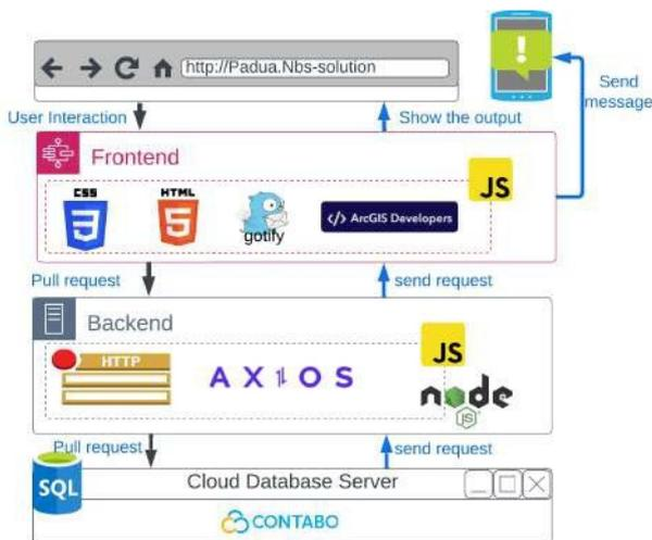
Figure 3. Architecture system design of the developed tool.
