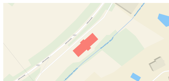
Figure 11. Visualization of the roof outline of updated Neuenburg model using IfcGref
