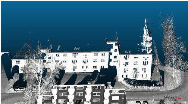
Figure 5. Reference point cloud of a building.
