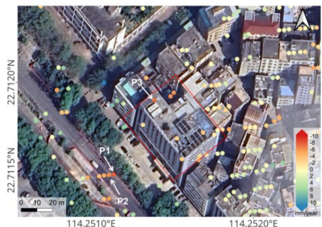
Figure 7. The red box denoting the Blueprint Hotel Garden shows the deformation rate results.
