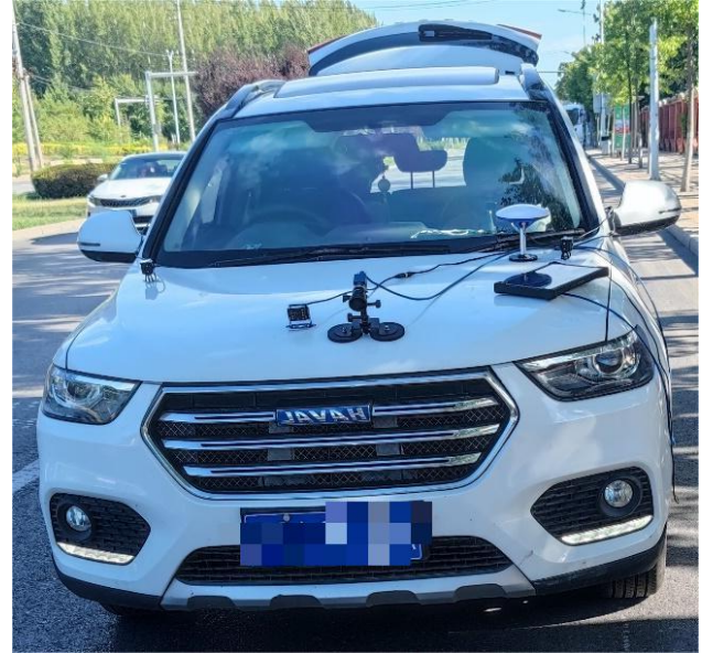
Figure 1 Construction of a lightweight collection system
