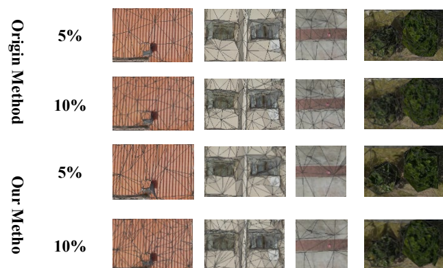
Figure 9. The figure shows the simplification results of the original method and our method for four classes at 5% and 10% simplification rates. From left to right are roof, building façade, ground, clutter
