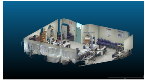
Figure 4. Fused RGB point cloud integrating Faro TLS and handheld RS10 data.
