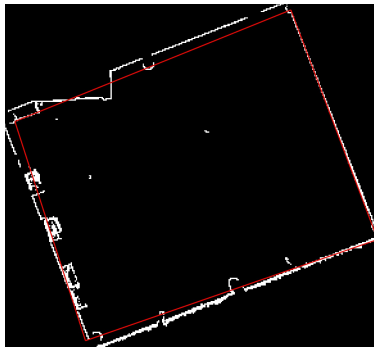
Figure 3. Orthogonal wall-line segments detected from the layered slices.
