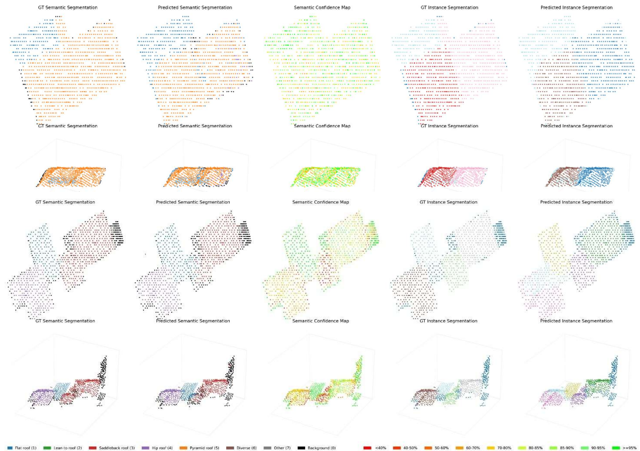
Figure 3: Illustration of segmentation and instance prediction results for two example cases. The figure includes: (a) noisy ground truth for segmentation (SemRoof dataset), (b) predicted segmentation, (c) confidence map for segmentation, (d) ground truth for instance segmentation
