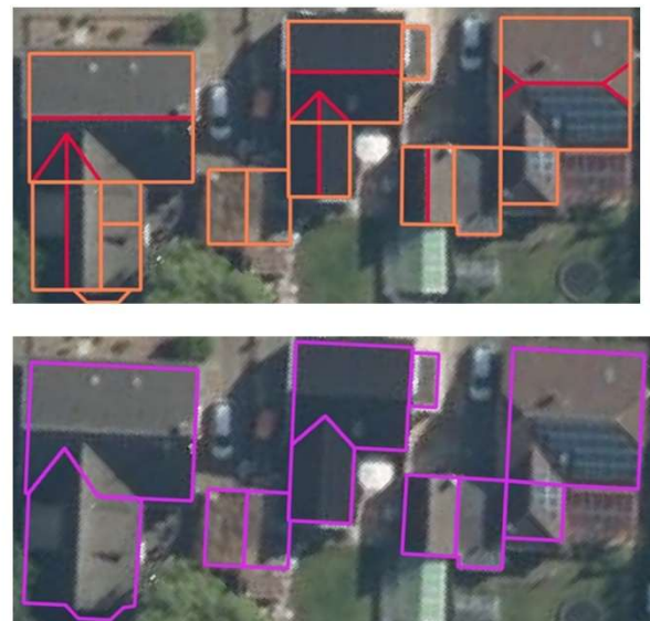
Figure 1: Top: Ground polygons (orange) and roof surface polygons (red). Bottom: Final roof part instance polygons (magenta) after refinement.
