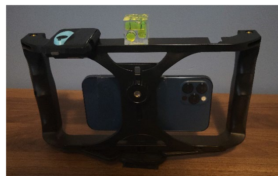
Figure 4. Smartphone rig with Apple iPhone 12 Pro and ZeroKey Quantum RTLS mobile node (at upper left).
