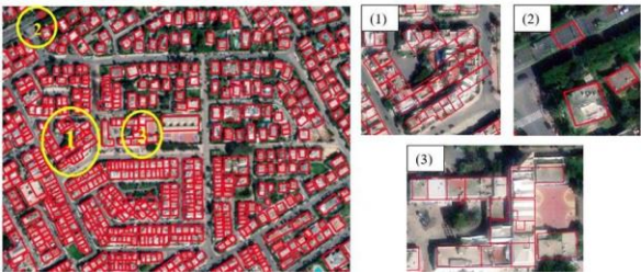
Figure 3: Result obtained by applying the "Mapflow" building model with an enlargement of visually detected anomalies.
