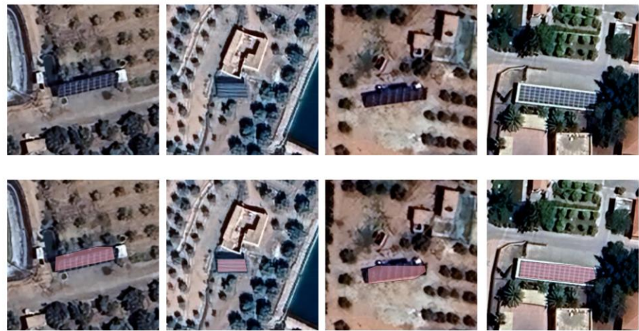
Figure 15: Different visual features of segmented PVs.
