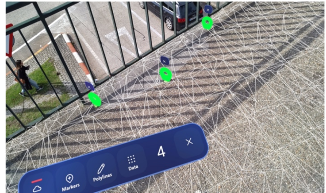
Figure 4. AR view of virtual tags, mesh and interface over real pedestrian pathway.
