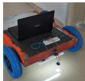
Figure 6. Tile material colour measurements conducted by the colour sensor assembled on the unmanned ground vehicle.
