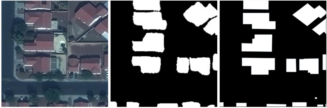
Figure 3. The result of the regularization process. First: input image. Middle: segmented image. Last: segmented image after the regularization process.
