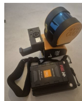
Figure 2. Image of the portable Mobile Laser Scanning (MLS) Zeb Horizon® by GeoSLAM adopted at the case study.
