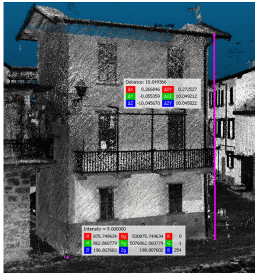
Figure 6. Reading coordinates of the volumetric unit's contour at ground level and the relative height by using the VRec approach and the SLAM Point Cloud.
