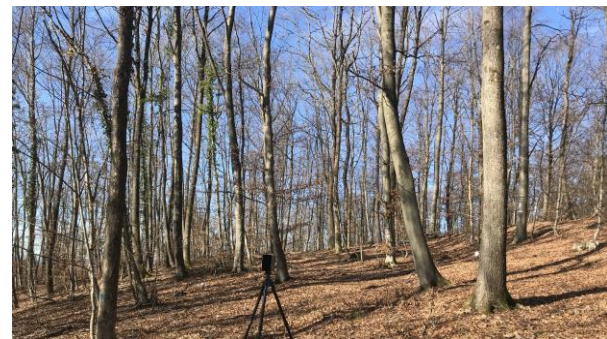
Figure 3. Static TLS using the FARO Focus M70 scanner on the European beech plot.
