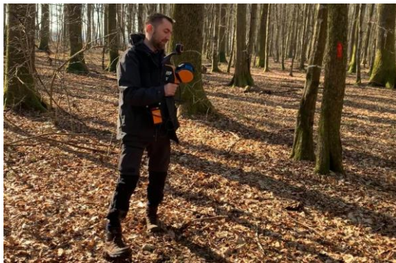
Figure 5. PLS survey using the GeoSLAM ZEB Horizon scanner on the pedunculate oak plot
