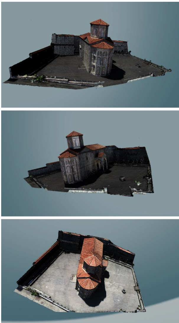
Figure 3. Web-optimized 3D model viewed from multiple angles. The model was processed in Blender using mesh decimation and exported in glTF 2.0 format for web compatibility
