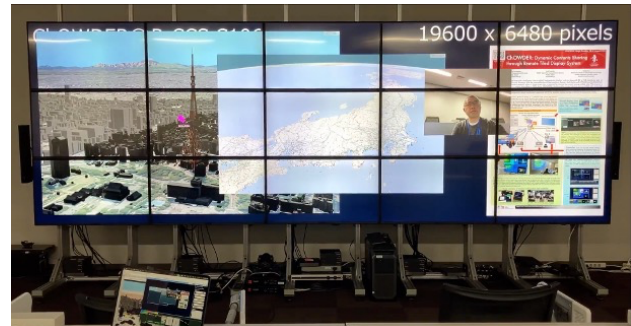
Figure 2. An example of displaying various types of content on a 20K horizontal resolution tiled display driven by ChOWDER.
